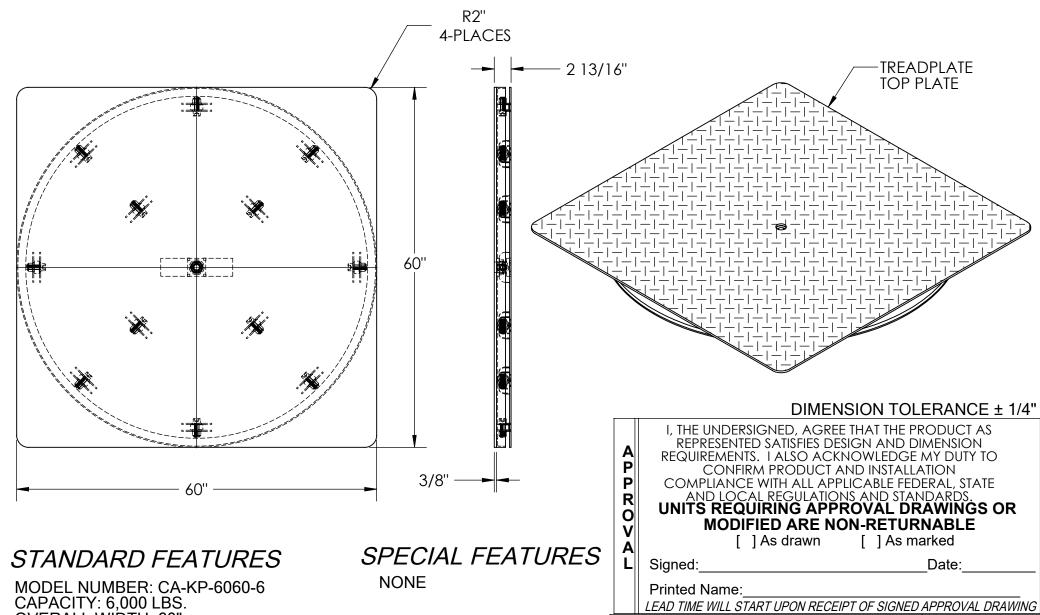
**OVERALL WIDTH: 60" OVERALL LENGTH: 60" OVERALL HEIGHT: 2 13/16"** SQUARE TOP TREADPLATE WITH ROUNDED CORNERS
